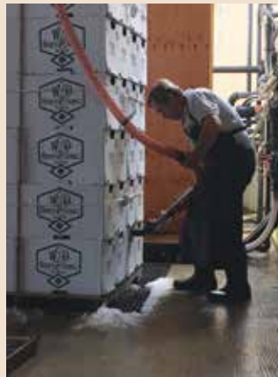
Given the variety of products produced and supplied by Eden Valley Growers, different cooling methods are required. This product receives an ice bath directly into the shipping box.
